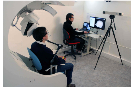
Fig. 2. The custom robotic system: the robotic device on the left, the software for the operator in the middle and the optical localizer on the right.
