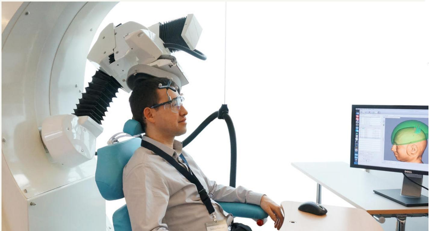
Axilum's TMS robot is operated by a computer and uses a stereoscopic camera (right) to monitor the slightest movements of the patient's head.
