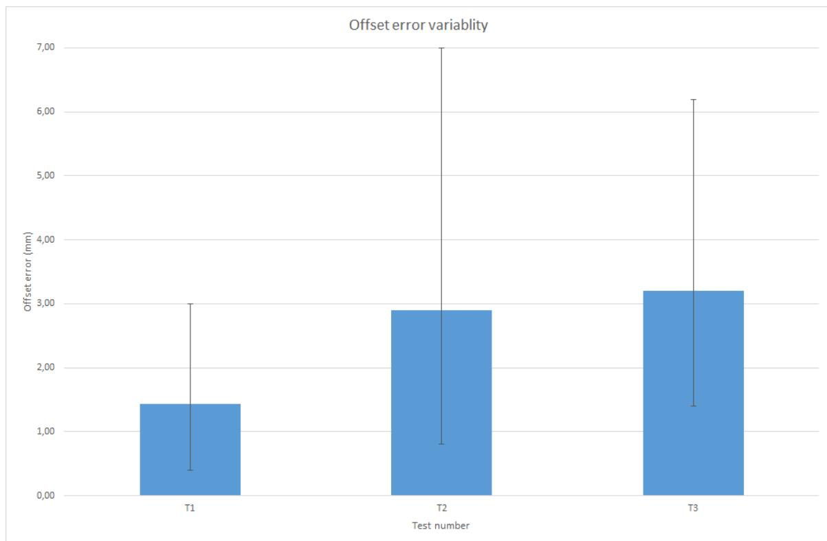
*Figure 2 - Offsets measured with the verification point in the 3 head registration tests.*
