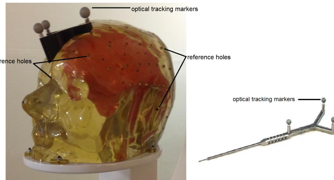
Figure 1 - Dummy plastic head equipped with optical tracking markers (left) and pointing tool (right)
